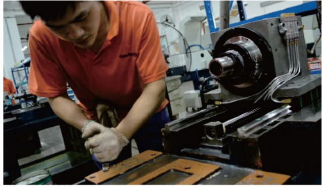
关键安装面铲刮修配 The scraper of main mounting surface
