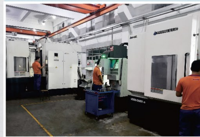
日本大隈卧式和立式加工中心 Japan OKUMA-BYJC Horizontal and vertical Machining Centers
