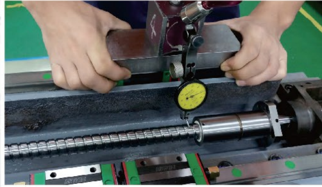
移动部件装配精度的再确认 Reconfirm the assembly accuracy of moving parts
